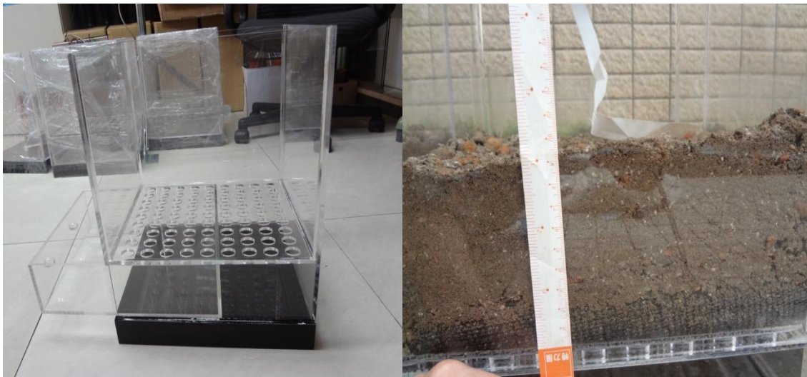
Figure 1. The left is the experimental container. At the bottom is a removal drawer to collect outflow water. The right shows the filter net and the substrate.
