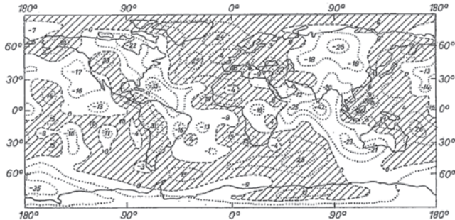
Fig. 1. Gravitational anomalies (in mgal) constructed from spherical harmonics up to 15th degree (Köhnelein, 1967)
